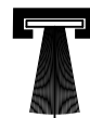
EC369A7145BL Aluminum T-slot extrusion with black pile insert, for bottom of doors
