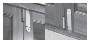
The flush-mounted flushbolts, rounded style and 1" (25mm) throw are designed for use with sliding and folding doors. This flushbolt will resist high winds and is rated to resist a 250kg load in Western Red Cedar and 450kg in Amoora. The bolts are easily installed with a dedicated router bit and are available in three finishes.
