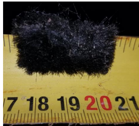
Pile dust pad used under each panel
